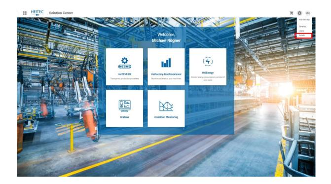
You are now in Asset Management. Note that in the following illustration, a site, a line and a machine have been created as examples. This hierarchy is very important for the operation of some applications and must be respected.
