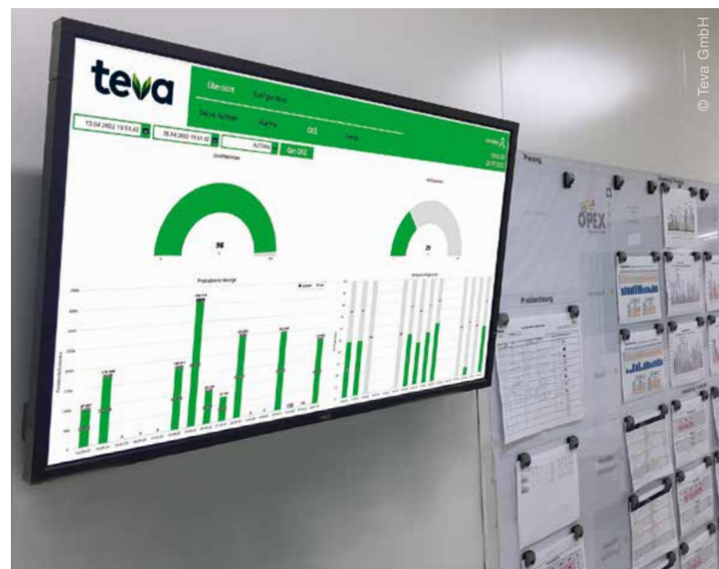
Production control is improved compared to earlier methods, thanks to the digital display of overall equipment effectiveness (©TEVA)
